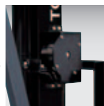
Lift-height Reel Sensor
